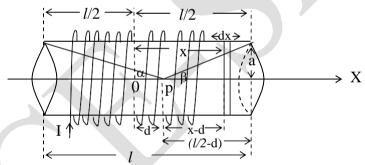
Let us consider a finite circular solenoid of radius 'a' and length 'l'. let 'n' be the no. of turns per unit length and 'I' be the carrying current. Assume that the solenoid axis coincides with the x-axis and the origin coincides with centre. Let 'p' be the point of observation at a distance 'd' from the centre.
