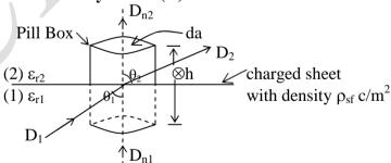
Consider a boundary formed by two dielectrics as shown in the figure. An infinite charged sheet with charge density  $\rho_s$  c/m<sup>2</sup> is placed at the boundary. The dielectric constants of the media 1 and 2 are  $\in r_1$  and  $\in r_2$  respectively.  $\theta_1$  is the angle of incidence.  $\theta_2$  is the angle of emergence.  $D_{n1}$  and  $D_{n2}$  are the normal components of flux density vectors.
