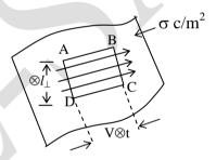
Flow of electric charges over a surface represents surface currents. Every surface current is associated with a mobile surface charge density  $\sigma$  c/m<sup>2</sup>.
