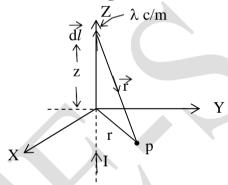
Consider an infinite straight conductor along the z-axis and carrying a current I along the positive Z-direction. Let 'p' be the point of observation on the x-y plane at a distance 'r' from the z-axis.
