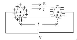
Current flowing through a conductor is directly proportional to the potential difference across it, provided temperature is kept constant.
