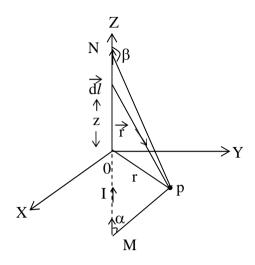
Let us consider a finite conductor of length MN, for the sake of generality OM  $\neq$  ON. Let 'p' be the point of observation on XY plane.
