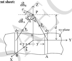
Let us consider an infinite current sheet lying on x-y plane carrying a surface current along the positive x-direction (  $\overrightarrow{K}$  ) with a surface current density K.
