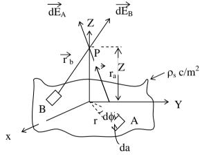
Consider two diametrically opposite elementary surface charges located at A & B. Let point of observation 'P' be along Z axis.
