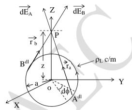
Consider two diametrically opposite elementary displacements located at A & B. Let point of observation 'P' be along 'Z' axis.
