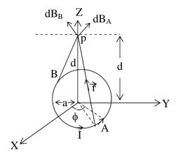
Consider a circular loop of radius 'a' lying on a x-y plane with centre at origin and carrying a current I as shown.
