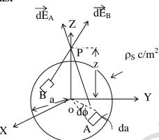
Consider two diametrically opposite elemental surface charges located at A & B. Let point of observation 'P' be along the z- axis.
