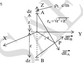
Consider an infinite line charge with a line charge density  $\rho_L$  c/m placed along the z-aixs. Let the point of observation 'P' be on x-y plane.
